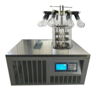
Manifold top press type (-80  $^{\circ}\mathrm{C}$ )
